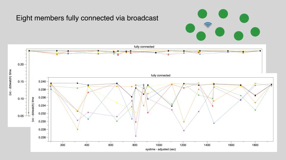
All 8 have the **same** offset after first calibration - the difference (max of 14ms) is just variations in the processing and capture times
